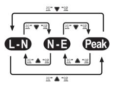
Voltage (V<sub>d</sub>): eal time display of cable connection status and display the voltage drop of current load and measurement results of phase voltage drop TRMS. This test item includes 3 submenus, namely load with 12A, 15A and 20A. Press Up "▲ "or Down "▼" selection key on the sub test item to enter the relevant test item.
